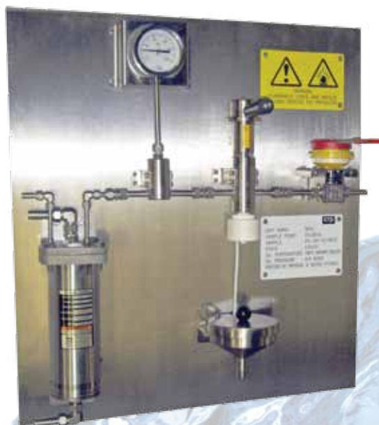
Panel mounted In-Line sample valve with In-Line heat exchanger to cool process media prior to it arriving at the sample valve, and temperature gauge.
