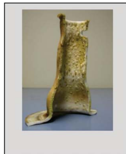
Typical permeation failure of isostatically formed liner
