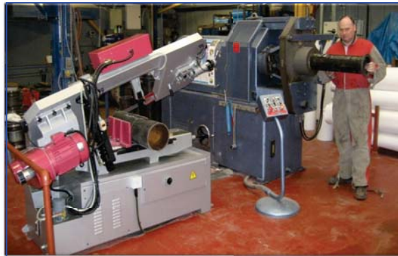
Van Stone Pipe Spool Manufacture
