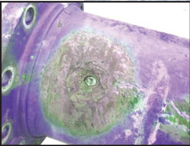
Corrosion of the vent hole area following permeation and no particular corrosion protection
